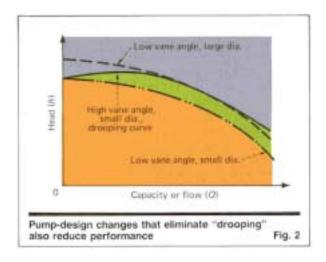
signed for optimum efficiency will tend to have drooping head-vs.-capacity curves. In pump terminology, pumps whose specific speed (N<sub>S</sub> = N( $Q^{1/2}/h^{3/4}$ )) is less than 1,000 will tend to have drooping head-vs.-capacity curves if they have an optimum number of vanes (7 or 8) and an optimum discharge angle (23 - 27 deg).
