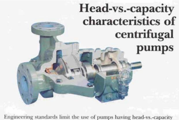
Engineering standards limit the use of pumps having head-vs.-capacity curves that do not rise constantly to shutoff. But in many cases such pumps are a good choice because of their high efficiency.
